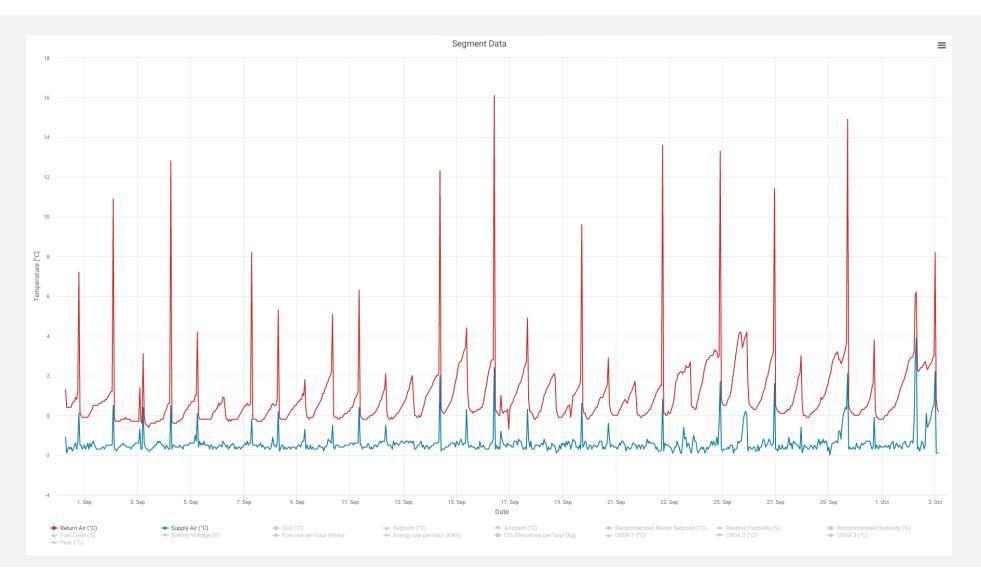
Here we see the a typical temperature chart from a marine container. The chart displays recorded air temperatures: supply air (blue) and return air (red). Neither of these air temperatures are a good estimate of the actual product temperature.
