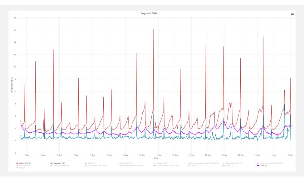
Here we see the same temperature chart, but with the addition of a product temperature sensor (purple). In this case a USDA temperature sensor. We can see that actual product temperature is not the same as either supply air temperature or return air temperature. Could it be possible to predict the product temperature using data such as air temperature readings from the container?
